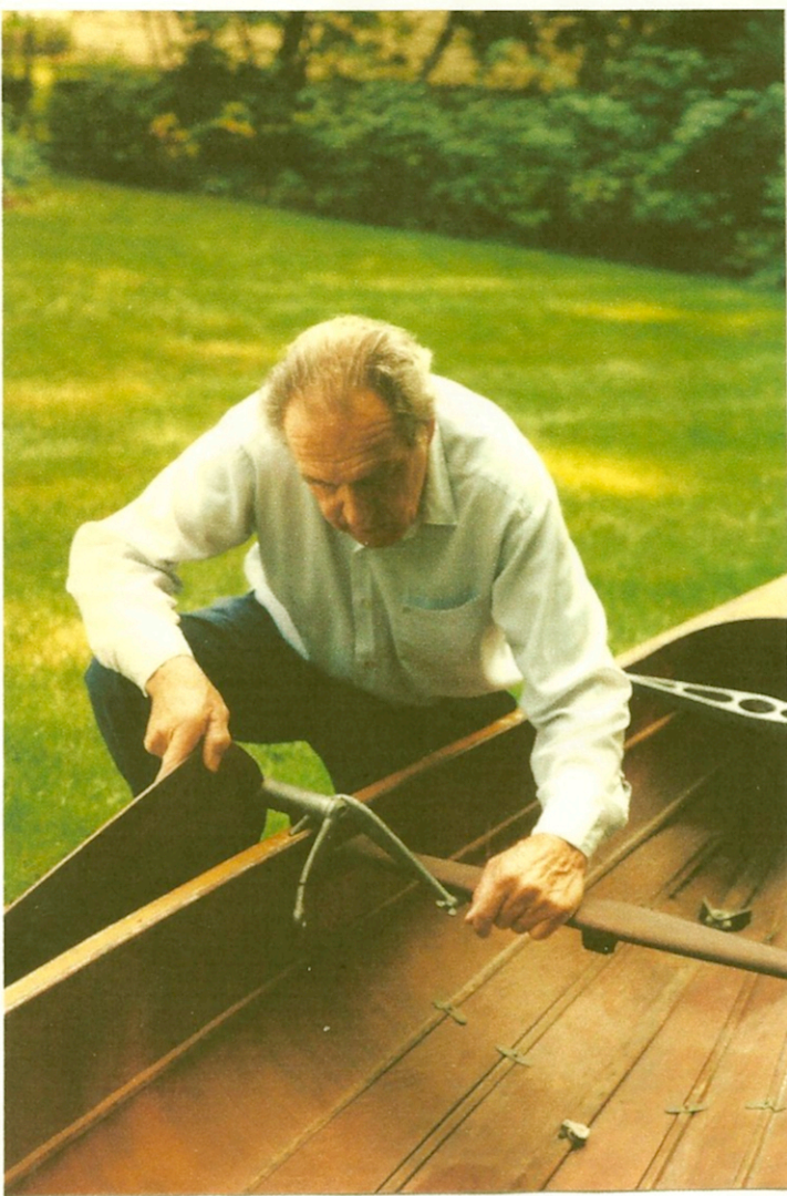
UNIQUE LEEBOARD MOUNTING Mounts on gunwale and thwart Spring loaded for adjustment with foot
