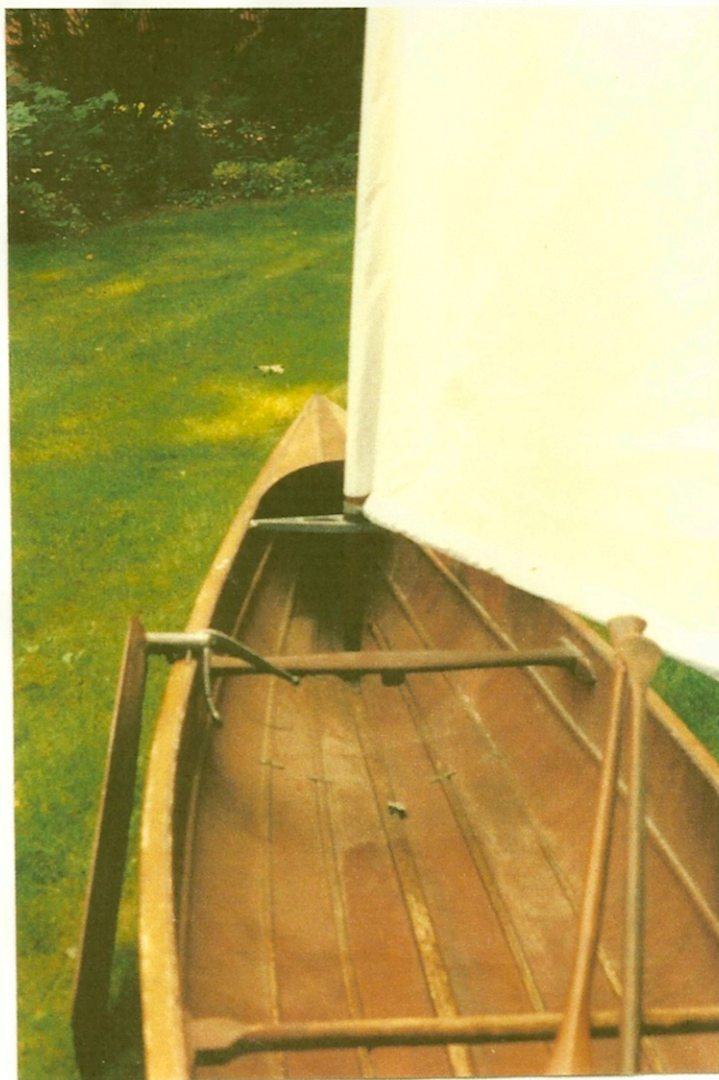
MAST THWART AND SLEEVE SAIL Specially cast mast thwart mounted to rotate up and down To hoist and lower entire mast and sail Very low boom and sleeve sail
